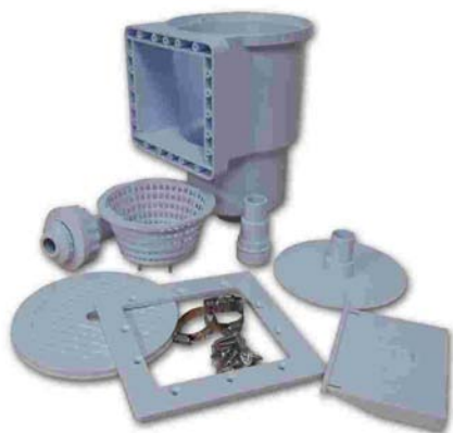
Ref. 4863 Skimmer completo: Cestillo, compuerta, racor, adaptador para barredera. Dimensiones de boca 14,8 x 14,1 cm. Full skimmer: Skimmer's basket, floater (door), hose's racor and an adapter to connect the hose. Skimmer complet: panier, porte, raccord du tuyau et un adaptateur pour connecter le tuyau.
